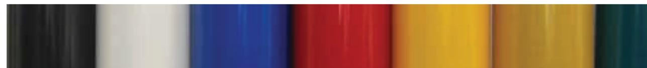
Vinyl is an inexpensive way to implement a sign system but generally do not last more than a few years in most exterior environments. Poor colors for a sunny environment include black, red, and green will get the most gradation and will be noticeably faded in 3 to 5 years. Protective surface treatment includes UV resistant clear coat that may extend the life of the solid colors by a few years.
