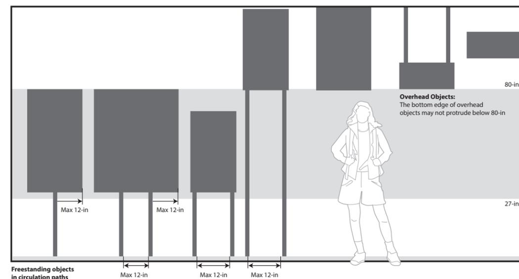
Minimum ADA clearances for protruding, overhead, and post-mounted objects
